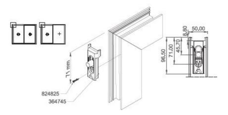
• The Anti-lift 291515 on the frame, above the top wedge
