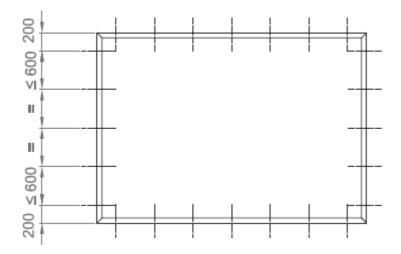
Secure fixings should be made through the frame (or on appropriate straps) at centres no greater than 200mm from each corner and 600mm intervals.
