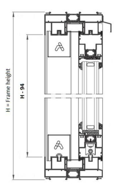
After fixing the frame in the structural opening and performing checks above, the sashes are carefully dropped onto the tracks.
